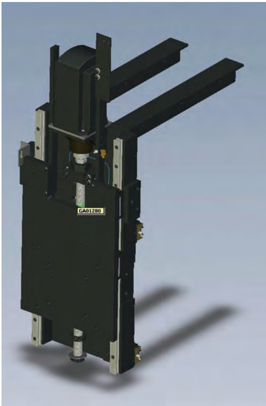
This is the image of the Z axis assembly that displays on your control screen for a CabinetShop 45.
