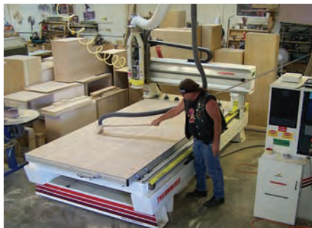
▶▶ Tom using overhead vac to clean handling sheet
