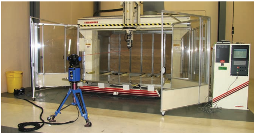
A typical set up to perform “volumetric compensation” on a five-axis CNC router.
