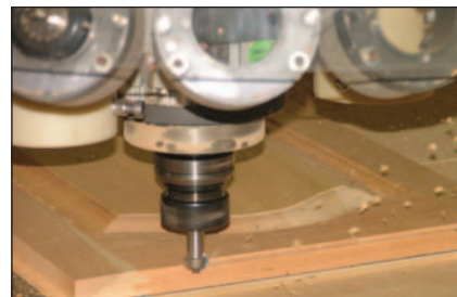
The outside edge is first cut with a straight bit and then the outside profile is added
