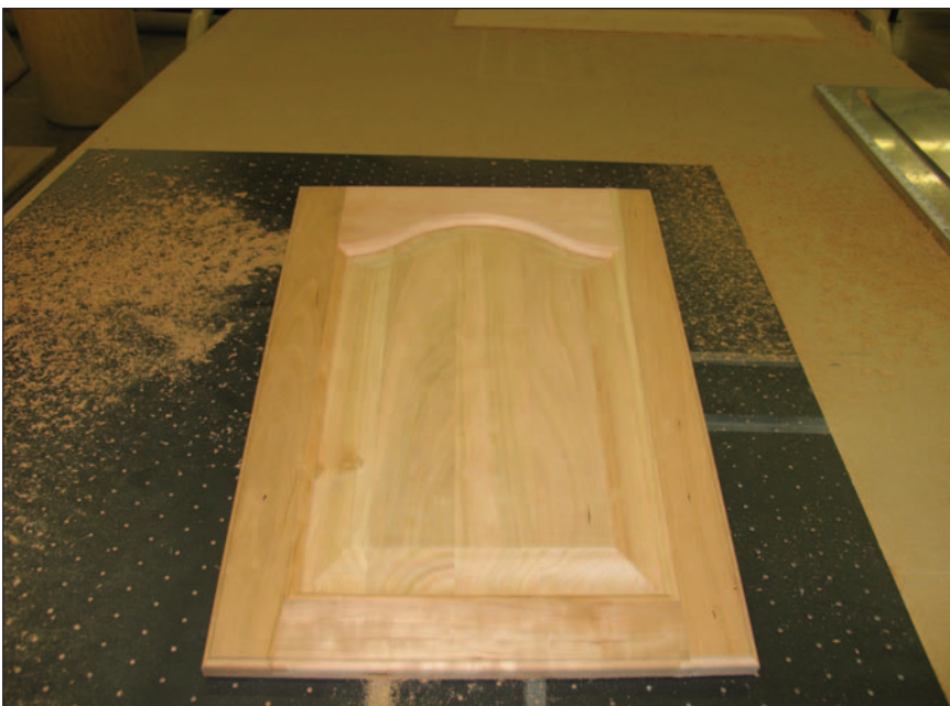
Center panel outline is first cut with a straight bit and then the raise is machined in several passes - all automatic
