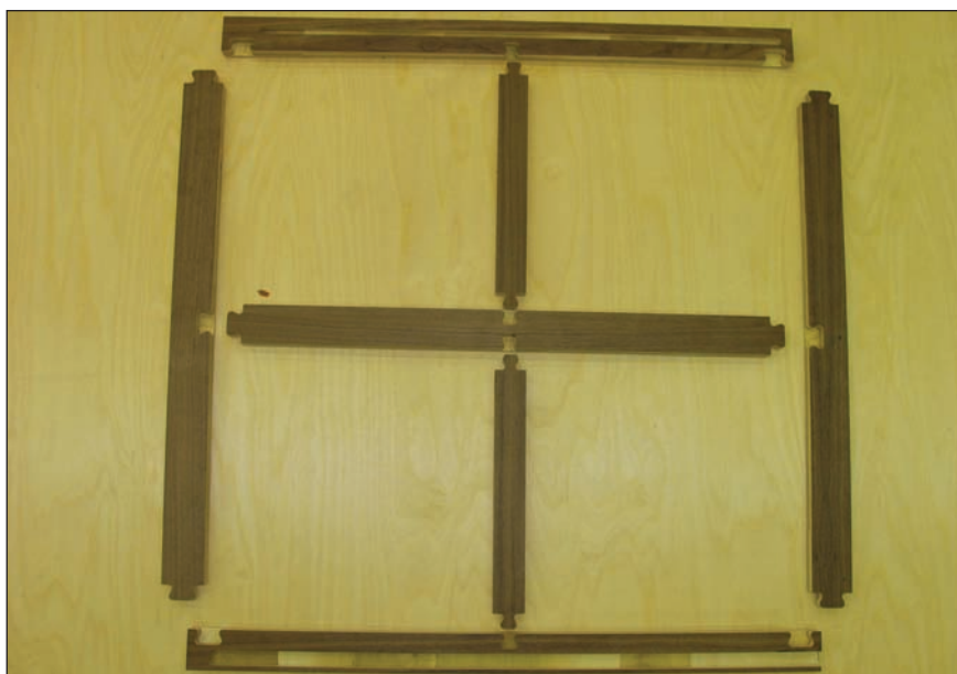
Puzzle joint face frame with mid stiles and mid rails
