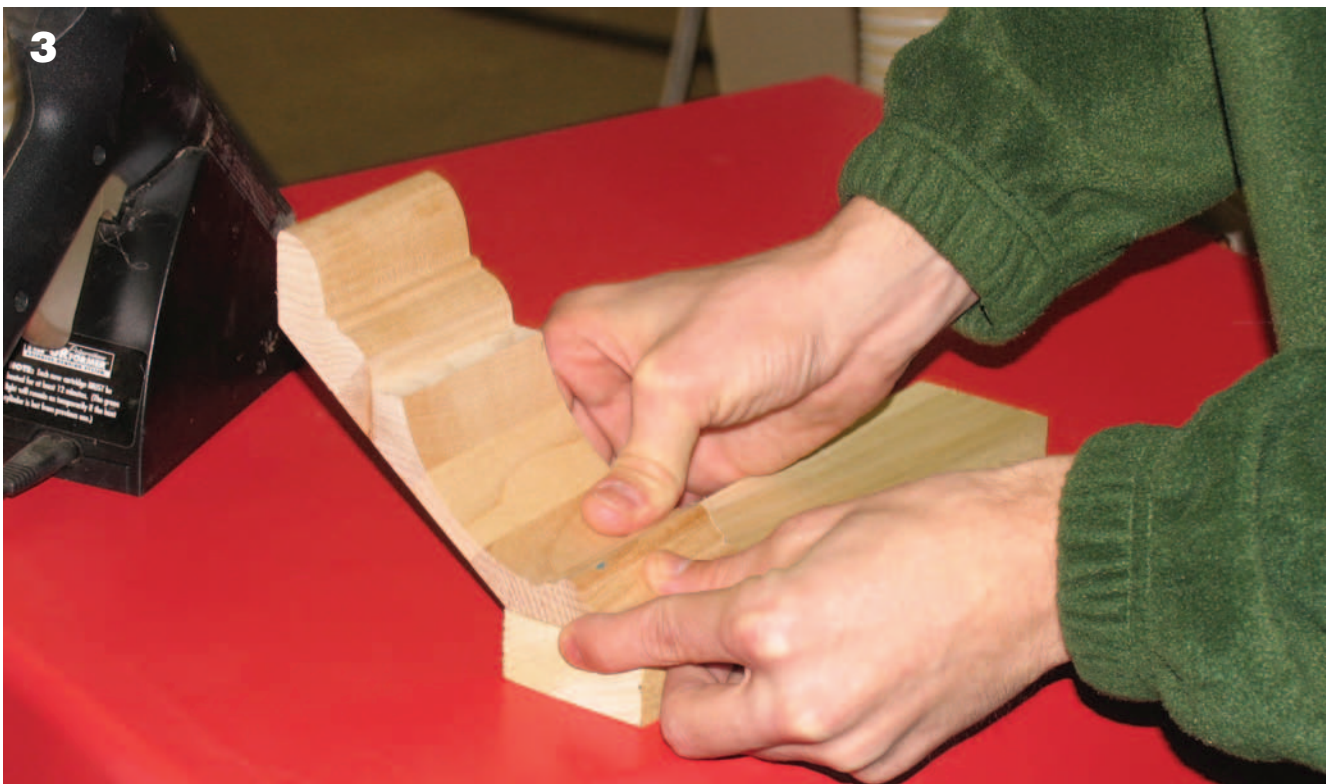
3 Hand pressure for a short time is all that is necessary for a permanent bond.
