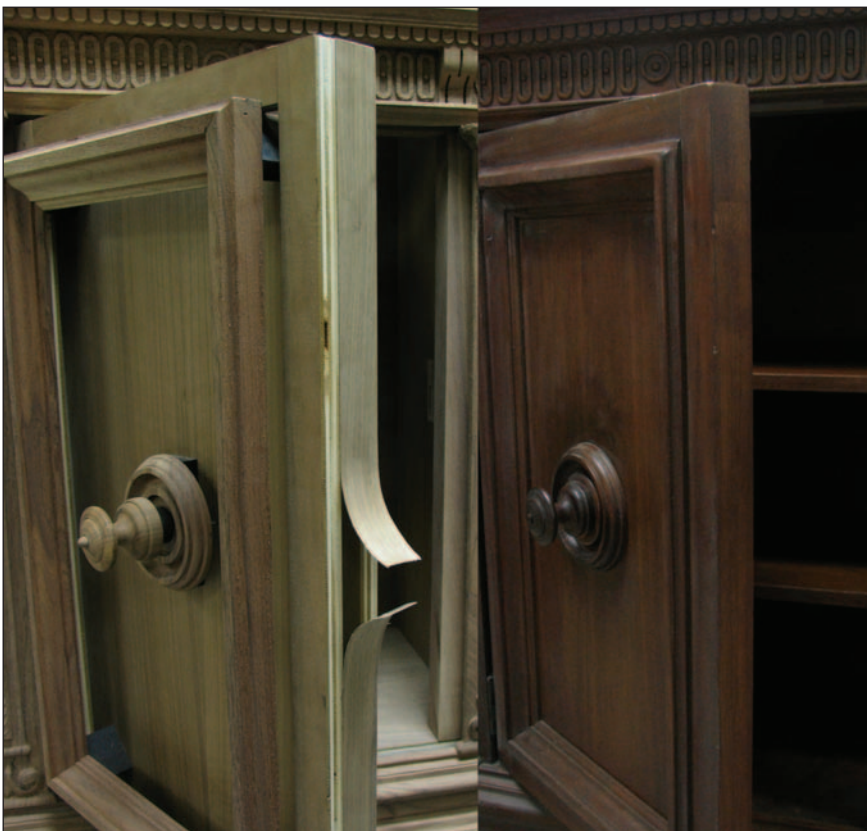
The Italian credenza door is made of walnut veneer plywood, a modeled center molding and walnut edge banding
